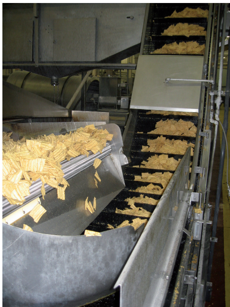
Inclined conveyor for chips for 2015 mattop chain
