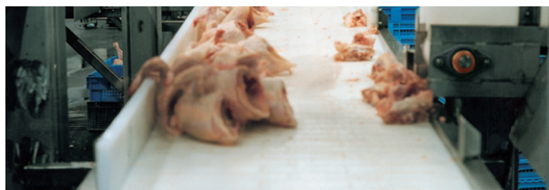
Chicken deboning line with 2015 mattop chain
