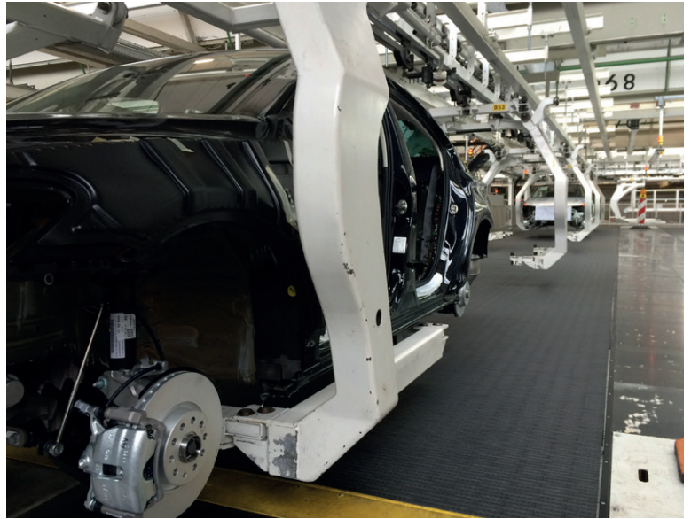
Conveyor equipped with Rexnord 1020 Series MatTop Chain
