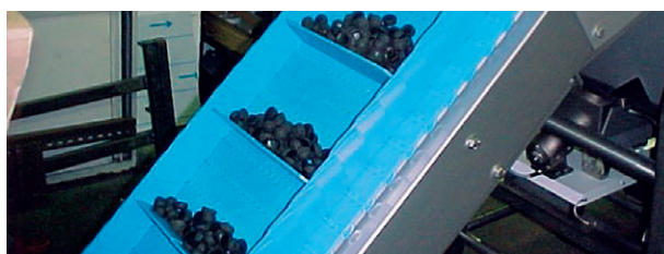
Confectionary elevating on 2015 mattop chain
