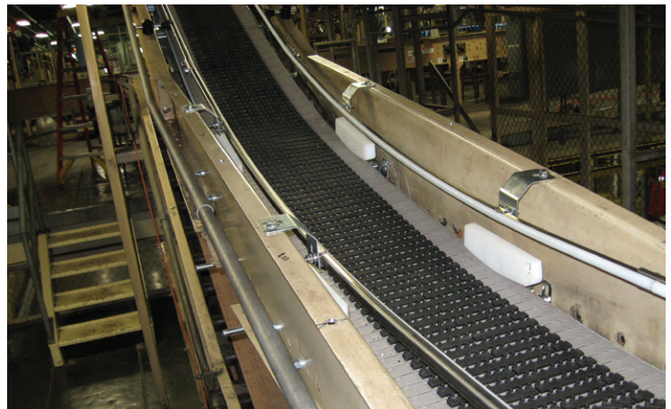
Conveyor with TCF7705 Belt
