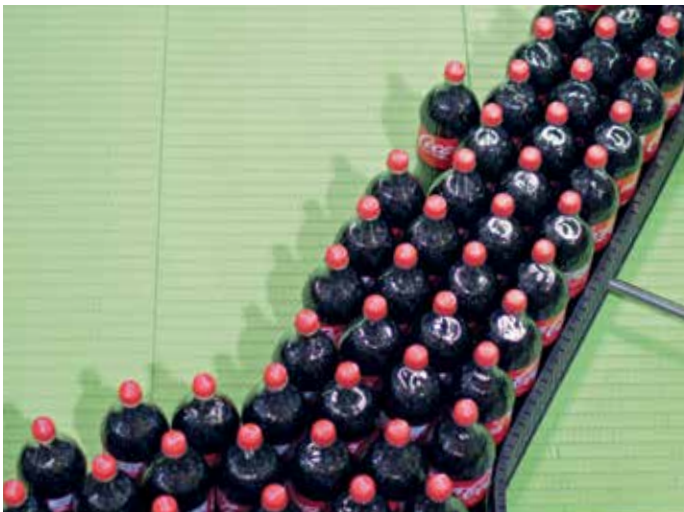
Bottle conveyor with FT1000 DRY-PT MatTop® Chain
