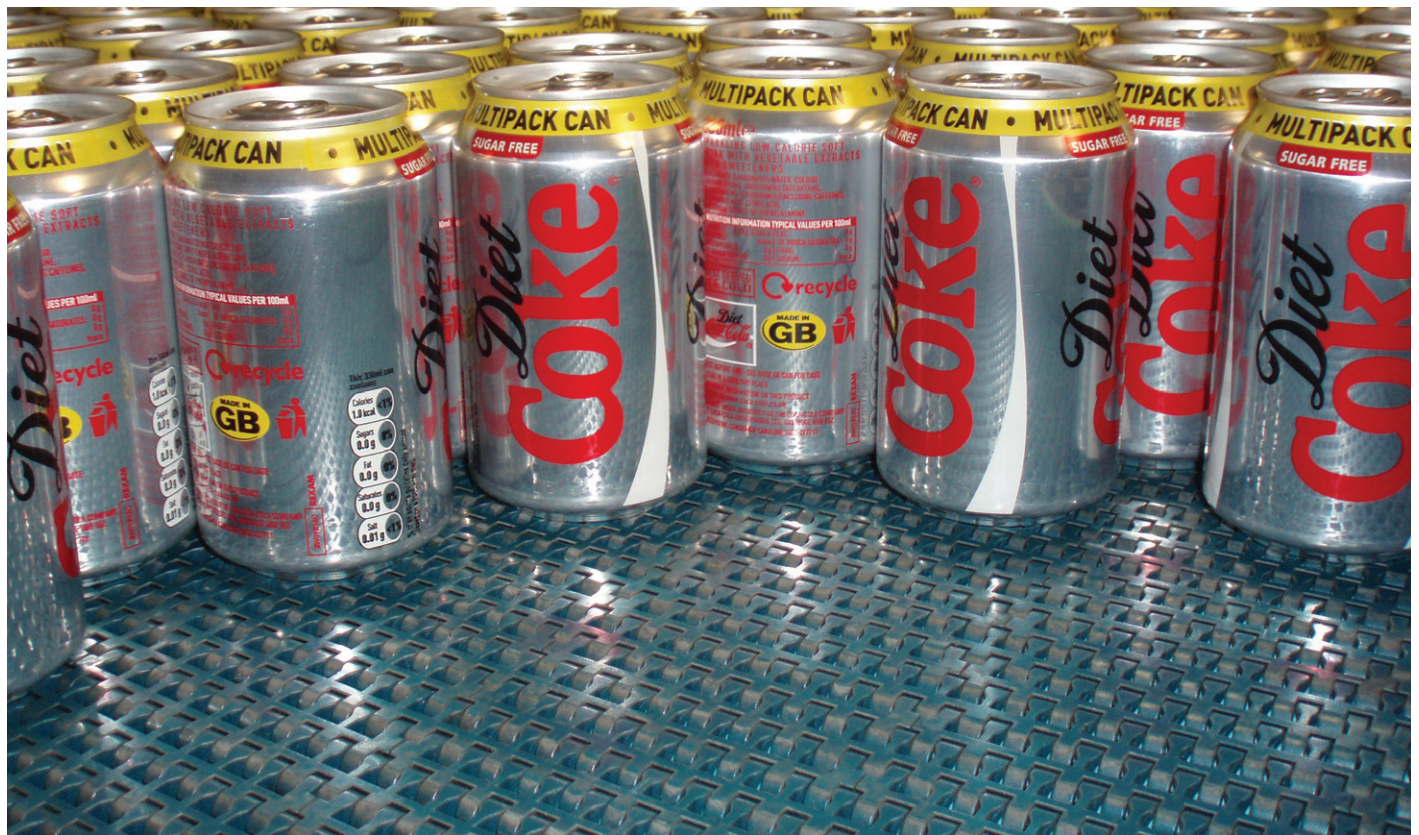
Conveyor with 500 belt.
