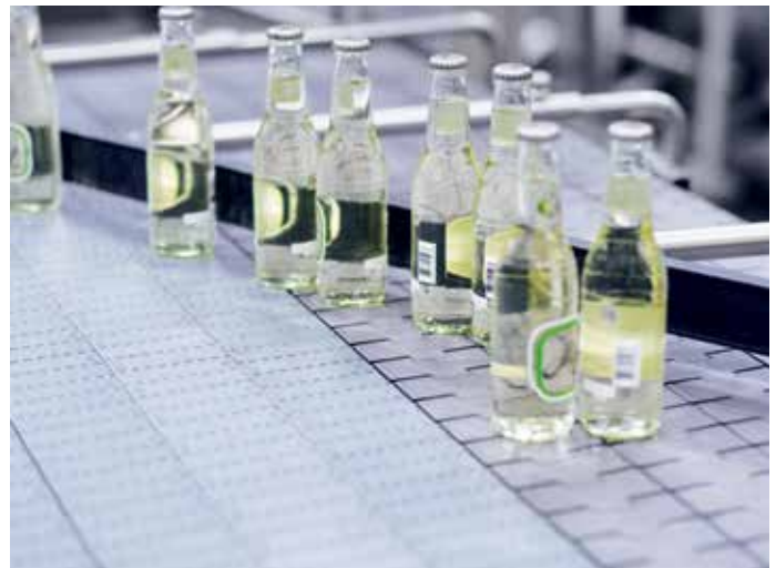
Bottle conveyor with FT1000 PSX MatTop® Chain
