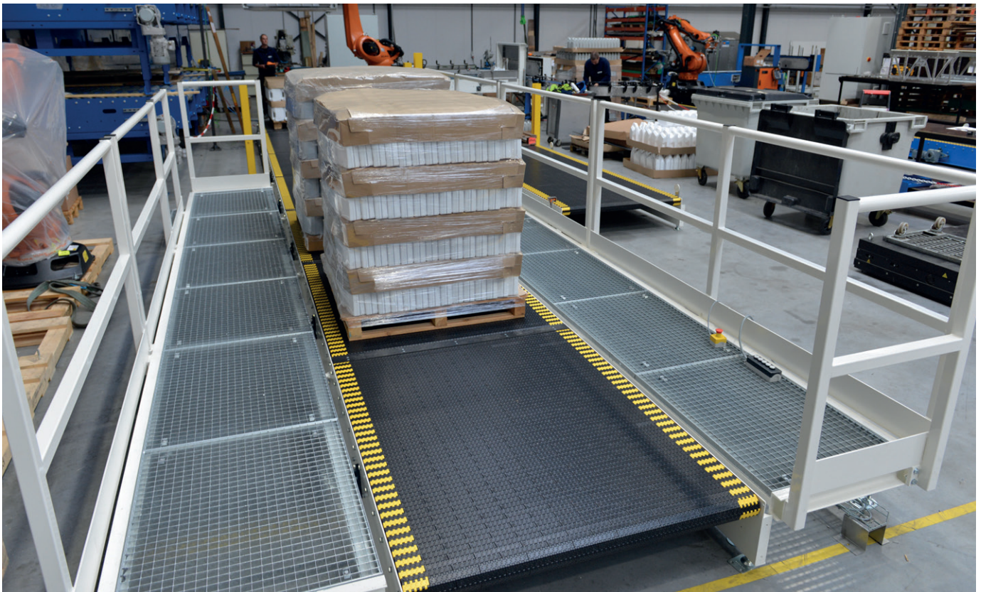
Conveyor equipped with Rexnord 1020 Series MatTop Chain
